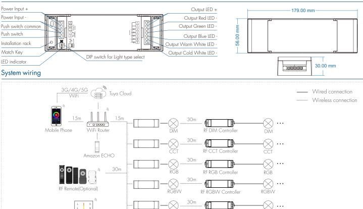
Note: 1. The above distance is measured in spacious (no obstacle) environment, please refer to the actual test distance before installation. 2. Please check if the WiFi router net in 2.4G band, the 5G band is not available, and do not hide your router network. 3. Please keep the distance between V5-L(WT) devices and router close, and check the WiFi signals.
