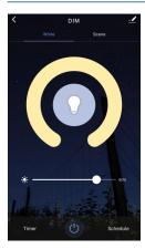
White interface For DIM type: Touch brightness slide to adjust brightness. For RGB type: Touch brightness slide, get RGB mixed white firstly, then to adjust white brightness. For RGBW type: Touch brightness slide, adjust white channel brightness.
